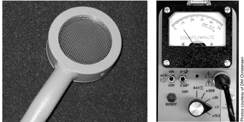
Figure 13.2: A pancake probe (A) is connected to the detection device containing the electronics for radiation detection and quantification (B). The numbers of radioactive disintegrations are tallied by the counter in counts/minute (cpm).
